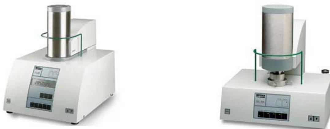
**FIGURE 2.9.** Photographs of the differential scanning calorimeters (i.e., STA Netzsch® 449C Jupiter and DCS Netzsch® 404C Pegasus) used during this study.
