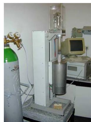
**FIGURE 2.5.** An altered vertical dilatometer (Bähr® DIL 802V and sketch of iridium indenter is shown on left.
