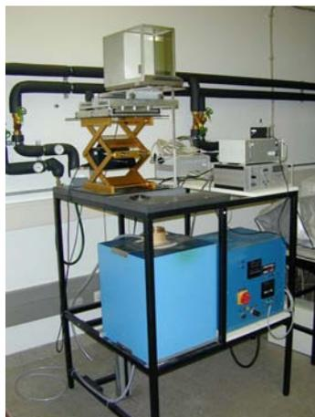
bob in the same manner. At the end of the last cycle the crucible containing the sample was removed from the furnace and quenched in water. A cylinder of glass 6 mm in diameter was drilled from this final product of the high temperature densitometry. Parts of this cylinder were then used for calorimetric and dilatometric measurements.
